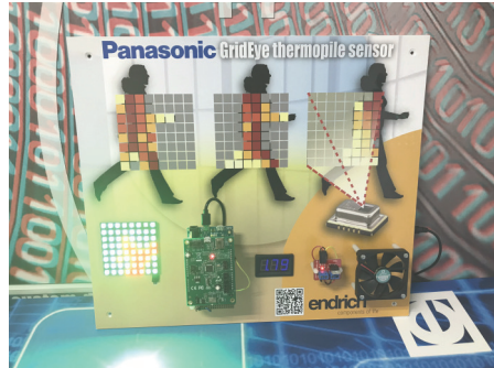
7| GridEye sensor controlled fan
